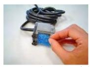
Once the cover has been removed, pull out the sponge-like filter and rinse it clean. With the cap removed, the impeller (the fanlike component) is accessible. The impeller
